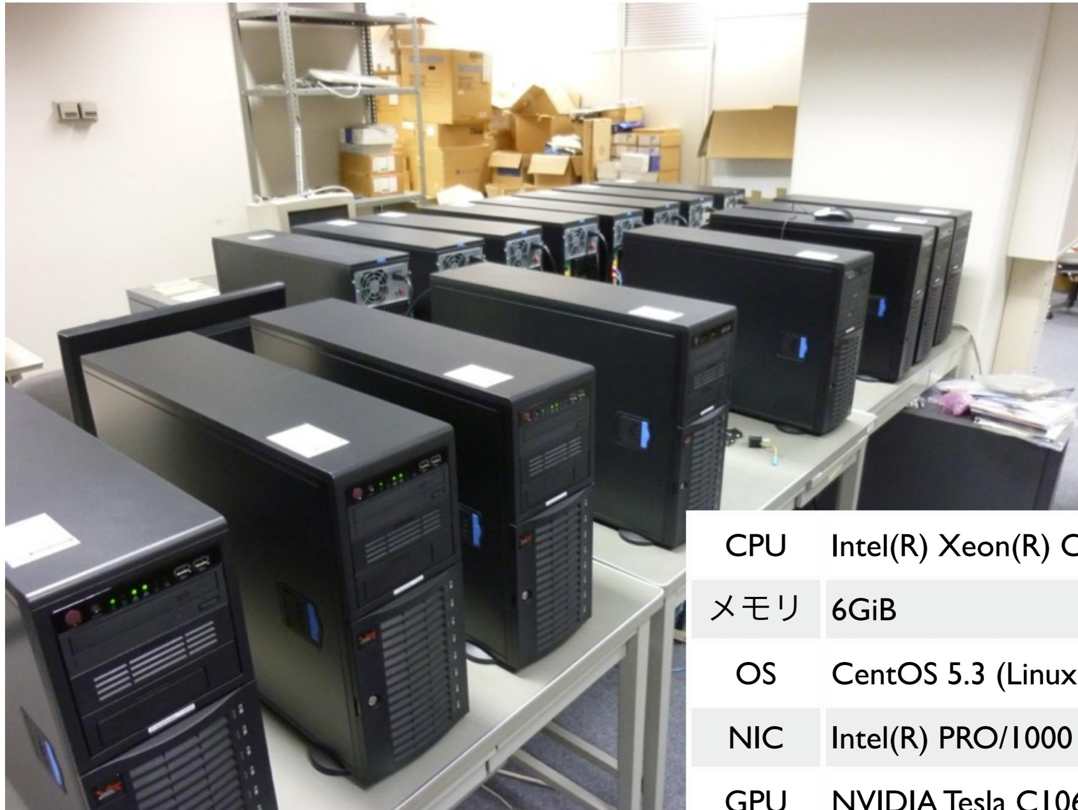
CPU Intel(R) Xeon(R) CPU W3520 2.7GHz
